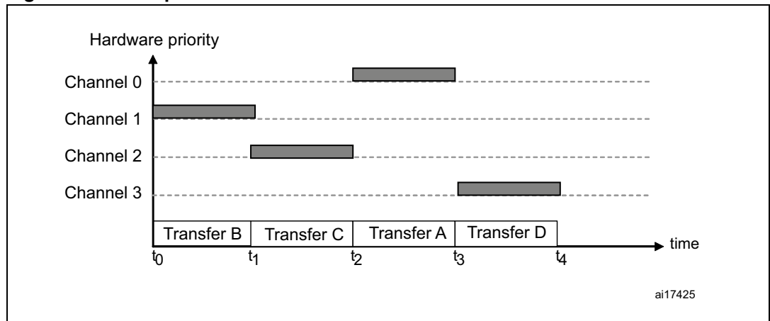
Figure 10. Example case 3: DMA channel data transfers as a function of time
