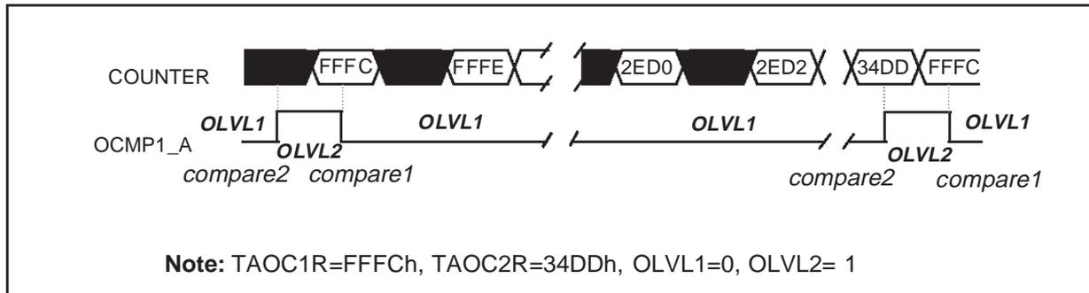
When you set the pulse length equal to the period in order to have a 100% duty cycle, you have a pulse of one CPU tick as shown in Figure 3. This could be useful for performing an external synchronization. However if you want a really 100% duty cycle you can use the TRUE routine described below.
