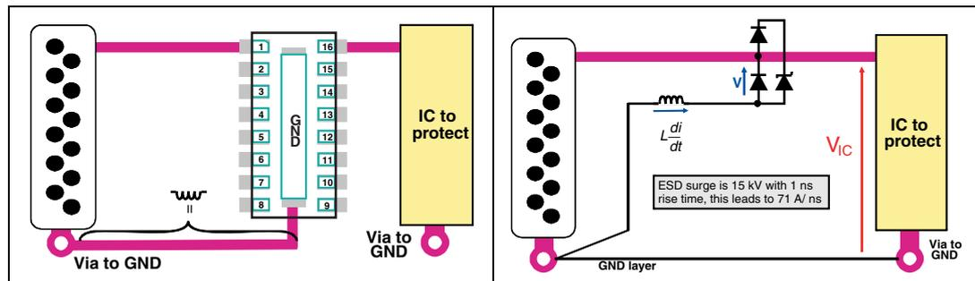
A very simple calculation shows that for a 15 kV ESD contact surge according to IEC61000-4-2, the overvoltage due to parasitic inductances may be really significant, as shown in *Figure 2*. This test is done with a contact discharge as the air discharge waveform is not defined in the IEC 61000-4-2 specification. Assuming that each inductance value is 5 nH (corresponds to metal track 5 mm long):
