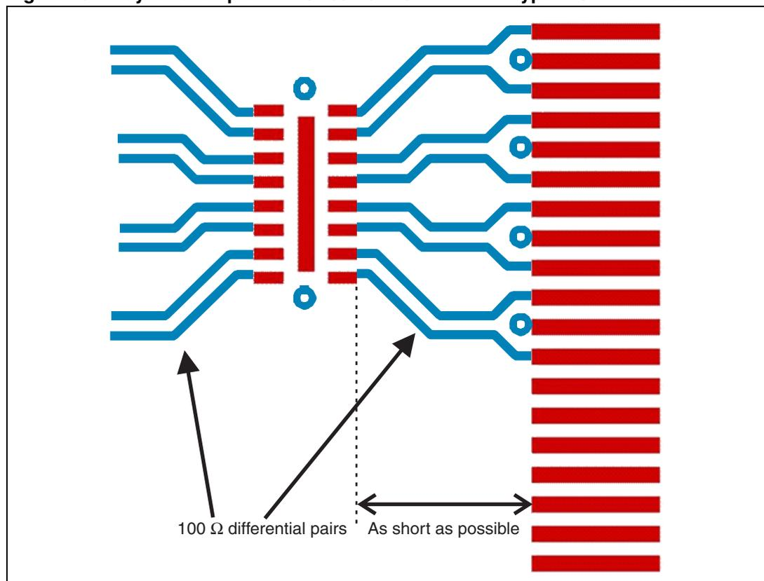
Figure 11 shows an example of PCB layout for HSP061-8M16 with an HDMI type C SMD connector
