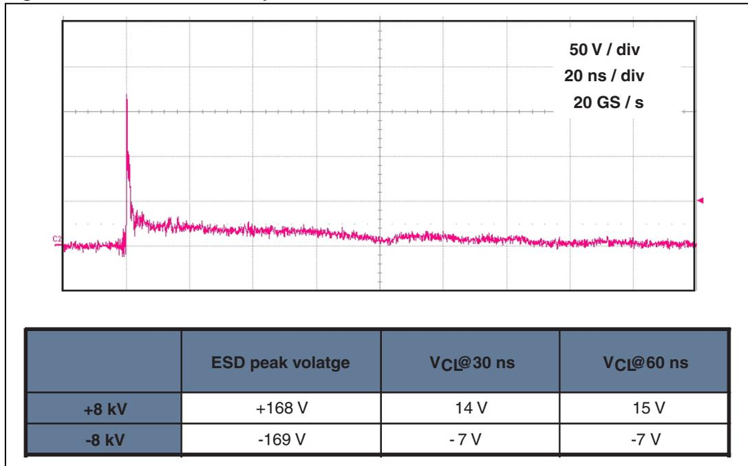
The goal of a protection device is to protect against parasitic disturbances. HDMI 1.4 standard specifies a 8 kV contact discharge requirement according to IEC 61000-4-2. The test must be performed 5 times with 1 second during each shot.
