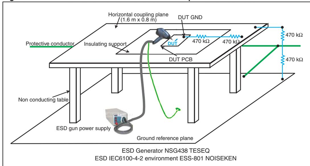
Our device is soldered on a dedicated PCB as shown in *Figure 3*. A 2 mm female banana plug is connected to the ground plane of the PCB. This plug, through the bleeder resistors (2 x 470 kΩ), links the horizontal coupling plane to the PCB ground plane.
