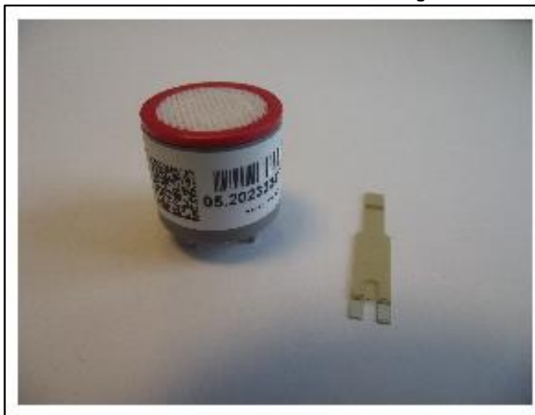
Figure 1: Electrochemical carbon monoxide sensor and glucometer test strip
