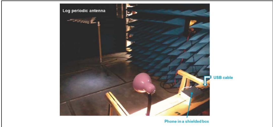
Figure 20. Radiated noise test setting (anechoic chamber view)
