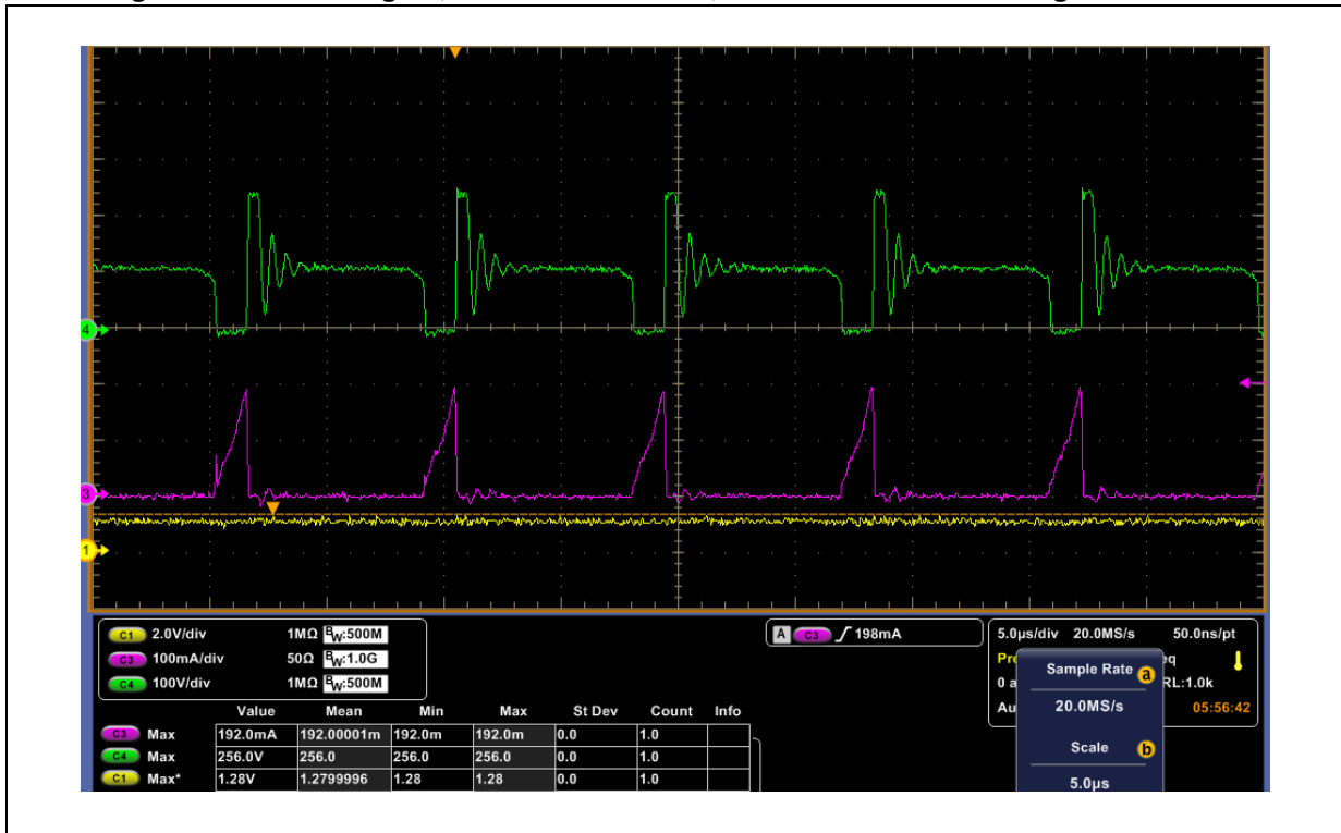
Figure 2. CH1: FB signal, CH3: drain current, CH4: drain source voltage at 100 VDC
