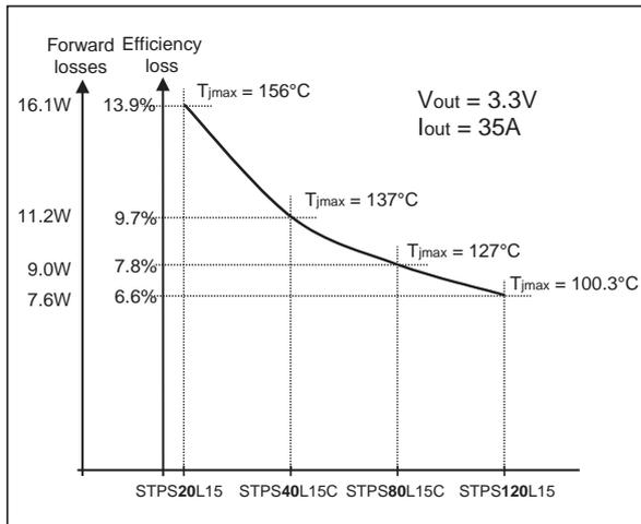
Using the specific thermal runaway law, the SMPS designer can optimize the OR-ing diode choice in order to improve the global efficiency.
