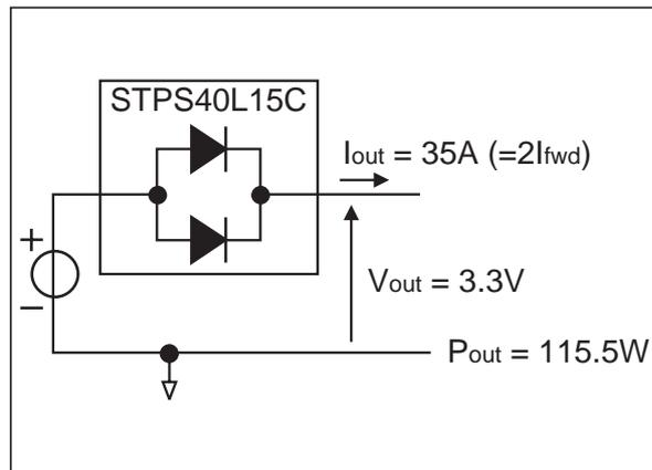
In the forward mode, the forward losses can be calculated as:
