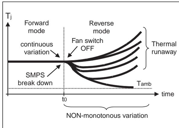
**Fig. 5:** Typical junction temperature variation in the OR-ing before and after the SMPS failure
