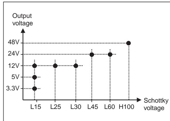
Using Schottky diodes provides very low forward losses. But the main important technology trade off for Schottky is between forward voltage drop and leakage current:
