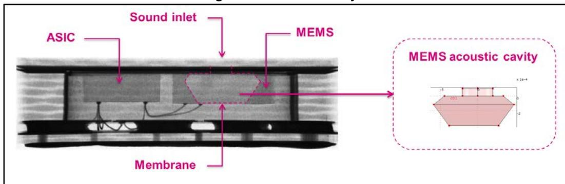
The first simulation performed with the COMSOL® tool represents the frequency response of the MP34DT05, applying 1 Pascal at the sound inlet and setting the silicon material properties as impedance boundary conditions. The tool solves the acoustic equations for every discrete point of the geometry and at the end of the simulation it is possible to plot the collected data in a relevant point. The evaluation point for the frequency response is one of the 4 corners of the MEMS membrane.
