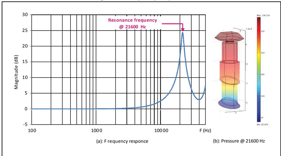
*Figure 12: "Frequency response"* (a) shows the frequency response characterized by a resonance peak around 21600 Hz; *Figure 12: "Frequency response"* (b) shows how the magnitude of the pressure, expressed in dB SPL, is distributed inside the cavity. The pressure inside the cavity is plotted at the resonance frequency; this is the reason why the maximum is exactly on the MEMS membrane.
