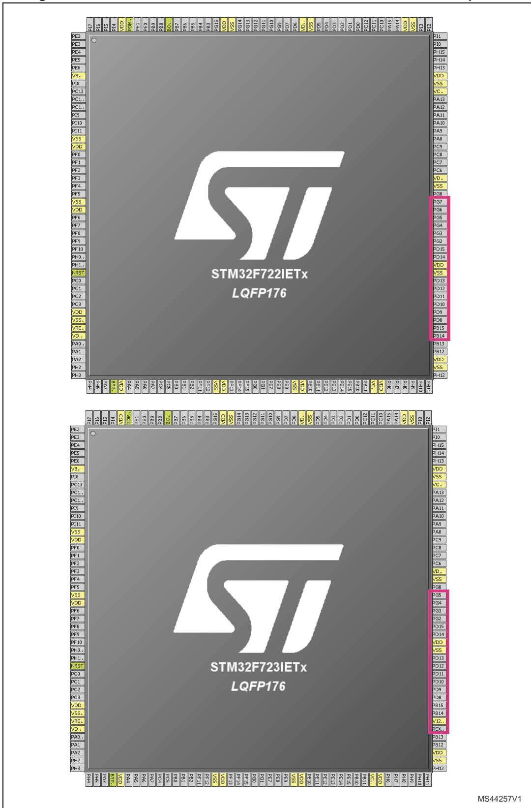
Figure 2. STM32F74xxx/F75xxx/F7x2xx versus STM32F7x3xx LQFP176 pinout
