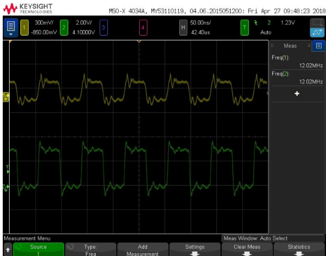
Figure 18. Receiver input and output waveforms
