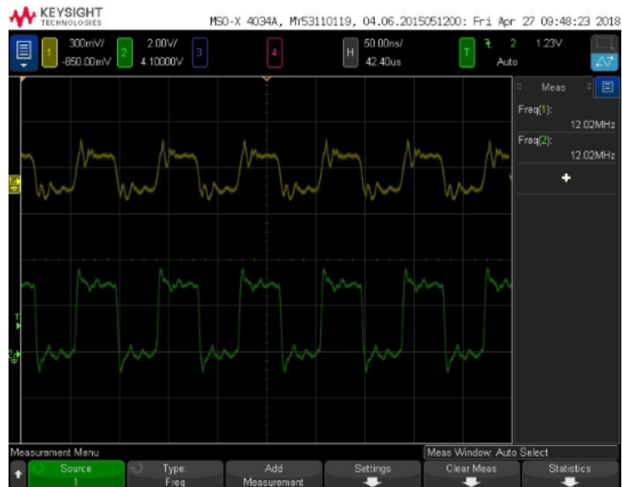
Figure 20. Comparator input and output waveforms
