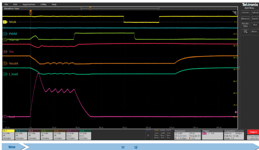
Figure 38. Unlatching sequence on HS
