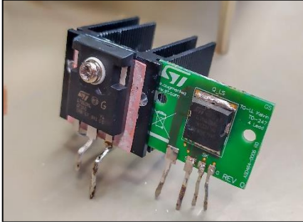
Figure 16 TO-247 with heatsink and TO-LL with daughterboard
