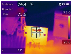
Figure 22 TO-LL temperature for the PFC section at 1.5kW of POUT
