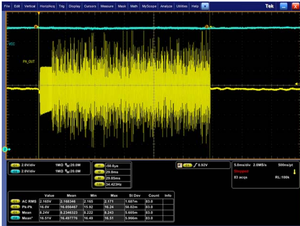
Figure 2. Output signal on PA_OUT pin vs. VCC supply level
