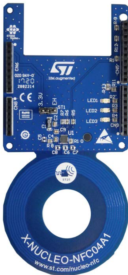
Figure 18. X-NUCLEO-NFC04A1 expansion board plugged to an STM32 Nucleo board
