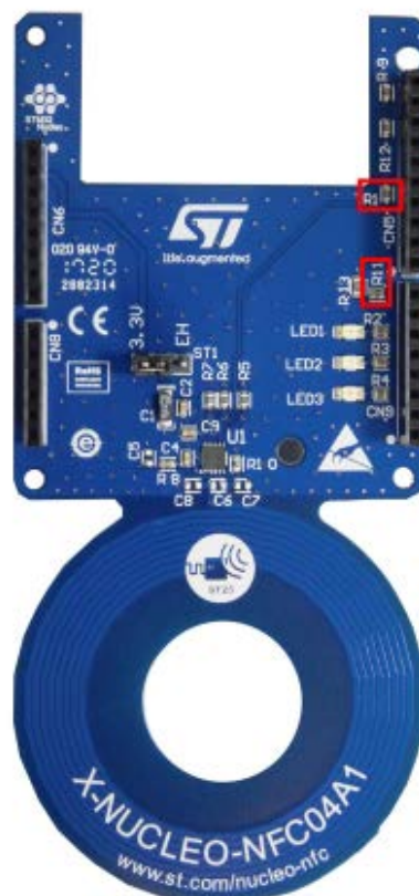
Figure 20. Modifications required for the X-NUCLEO-NFC04A1 expansion board
