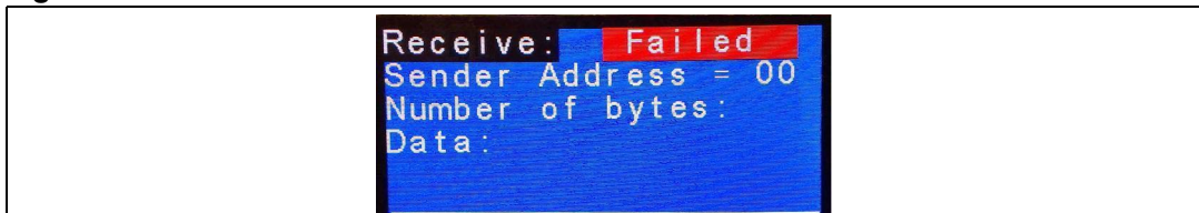
Figure 11. LCD screenshot of a failed receive transaction
