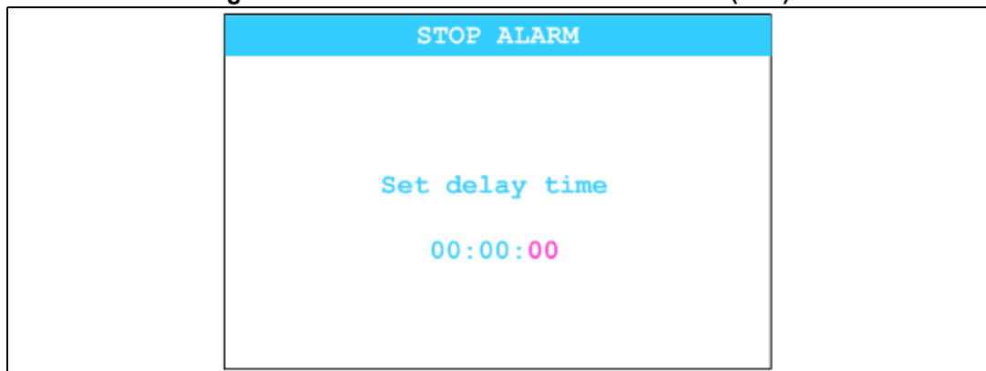
Figure 49. Exit from STOP mode - RTC Alarm (WFI)
