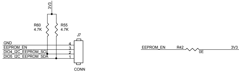
Figure 7: STEVAL-BLUEPLUG1 schematic - M24LR dual EEPROM
