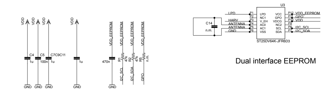
Figure 3: STEVAL-SMARTAG1 schematics - voltage regulator, battery holder and EEPROM
