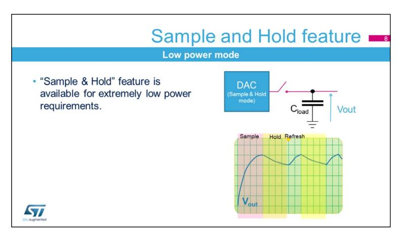
The digital-to-analog converter has a Sample & Hold mode feature. The DAC can work intermittently, charge the external or internal capacitor, and be powered down while the output voltage is kept on the hold capacitor. After a certain period, the DAC is powered back on again and recharges the hold capacitor.
