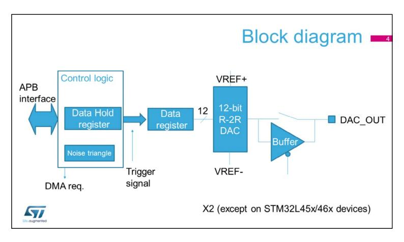
Here you can see the simplified block diagram of the digital-to-analog converter. The STM32L4 integrates 2 of them except on STM32L45x/46x devices were only 1 DAC is implemented.
