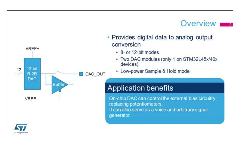
The digital-to-analog converter on STM32L products ensures the conversion of 8- or 12-bit digital data to the analog voltage. Two DAC modules are embedded in the STM32L4 devices, except on STM32L45x/46x devices were only 1 DAC is implemented.
