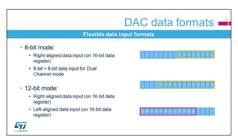
The DAC can support different input formats. In 8-bit mode, it's a right-aligned 8-bit data format. In Dual channel mode, it's an 8 bit plus 8 bit data format, in order to provide input data for two DAC simultaneously. In 12-bit mode, either a right- or left-aligned mode can be used for input data.
