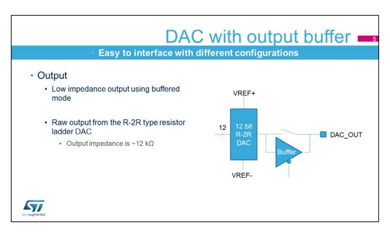
The DAC output can be buffered for low impedance loads. When unbuffered, the output is directly connected to the R-2R resistor ladder network type of DAC.
