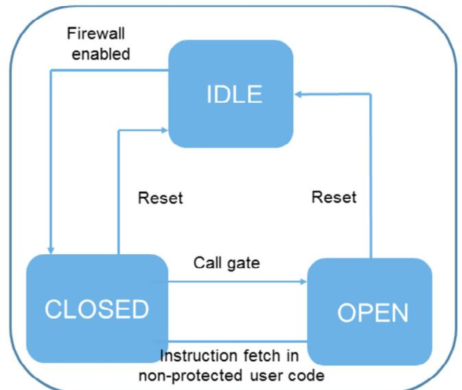
The Firewall is based on 3 states to ensure a dynamic protection of the secure segments. The Idle state is the default state when the Firewall is not enabled. In this state, the AHB memory bus is not monitored. When enabled, the Firewall enters Closed state and all access to the protected segments is prohibited.
