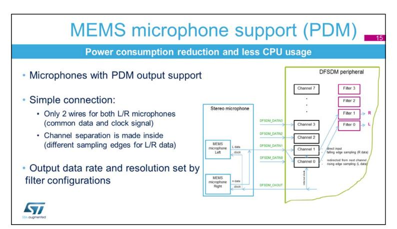
The MEMS microphone provides a pulse density modulated (PDM) data signal whose format is theoretically like the Sigma-Delta bit stream from Sigma-Delta modulator.
