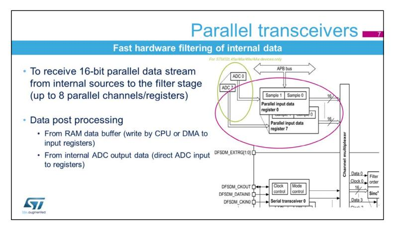
Parallel transceivers provide parallel inputs from internal data sources; for example, from memory buffers.
