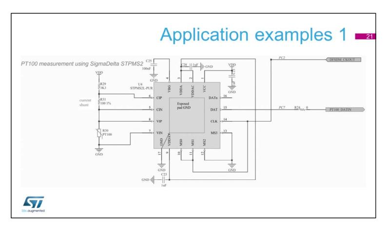
This schematic shows an example of the Pt100 thermometer. Here you can see how the STPMS2 device senses the voltage and current over the Pt100 sensor. Sensed data are sent from the STPMS2 device to the DFSDM peripheral through the serial interface.
