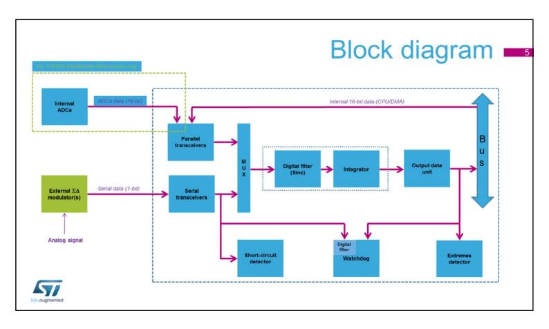
The entire Digital Filter for Sigma Delta Modulators interface consists of:
