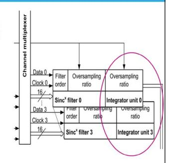
The Integrator unit performs additional simple averaging of data provided by the digital filter. It provides just a simple summing of the data coming from the digital filter. The number of samples to be summed can be set from 1 to 256. The correct configuration must take care that the final data length fits into the 31-bit width, which is the resolution of the internal integrator. The width of the data coming from the digital filter must also be taken into account.
