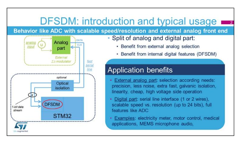
The DFSDM Peripheral is a new digital peripheral inside the STM32 products. Its behavior is finally like standard ADC with the analog part outside the microcontroller.
