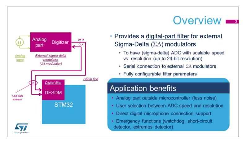
The DFSDM was developed due to need for a sigmadelta ADC with scalable speed vs. resolution.
