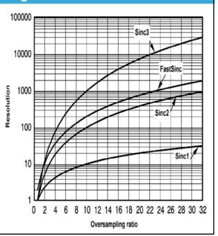
The digital filter averages the 1 bit input data stream from the Sigma-Delta modulator into a higher resolution, but with a slower data output.
