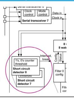
The short-circuit detector monitors input serial channels for a saturation state. When an input signal is saturated, it means that it is outside the allowed measurement range and therefore there is an overflow or underflow of the signal. When measuring current, this event usually detects an overcurrent (or short circuit), or an overvoltage when measuring the voltage.
