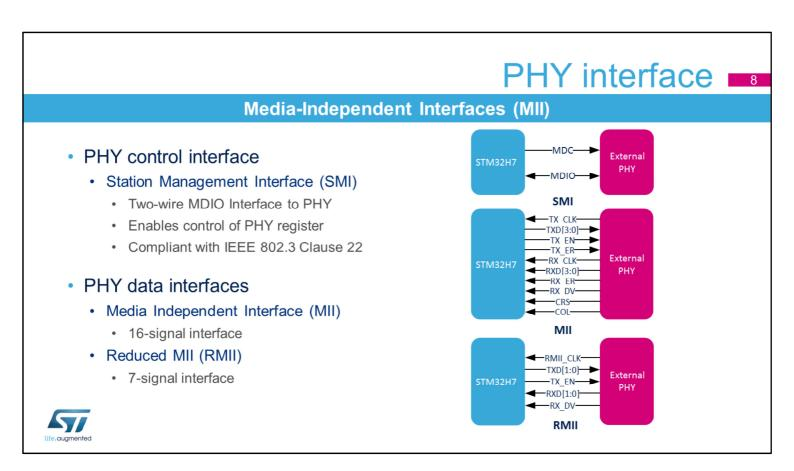
The external PHY is controlled by the peripheral through the Station Management Interface (SMI) that allows read and write access to PHY internal registers. This interface supports the MDIO protocol on a pair of wires. Read and Write operation codes are available.
