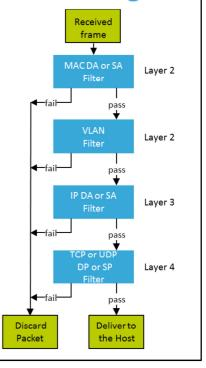
The Ethernet MAC peripheral offers some filtering capabilities that can be applied to the received frames. The different filters are nested. Layer 2 is filtered first with the MAC addresses and VLAN tags; then the Internet layer's filter is applied based on IPv4 or IPv6 addresses; and finally, frames are filtered following the port number of UDP and TCP protocols. Any frame rejected by one of the active filters will be discarded and not delivered to the Host.
