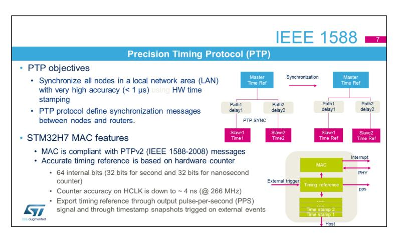
The precision timing protocol has been developed to support high-precision synchronization between several nodes of an Ethernet network. The targeted precision is approximately 1 µs. This level of precision can only be achieved by hardware support for packet time-stamping.
