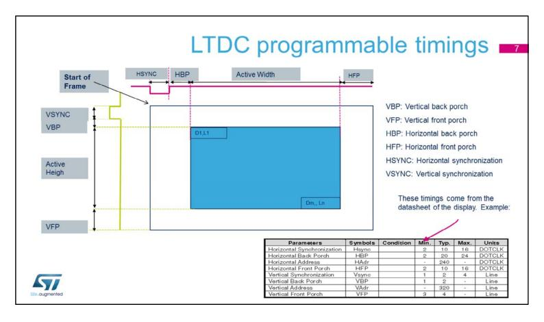
To interface with TFT panels, all timings are programmable through the LTDC controller. These timings come from the TFT panel datasheet and are:
