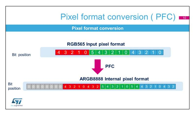
When the color format of a bitmap is converted into another one, this operation is called Pixel Format Conversion (PFC).
