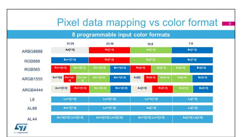
The programmable pixel format is used for the data stored in the frame buffer of a layer.
