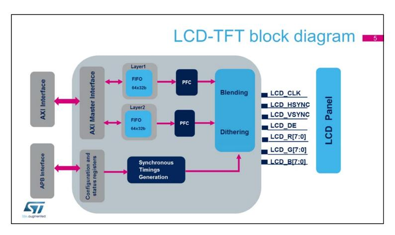
This is the LCD TFT controller block diagram.
