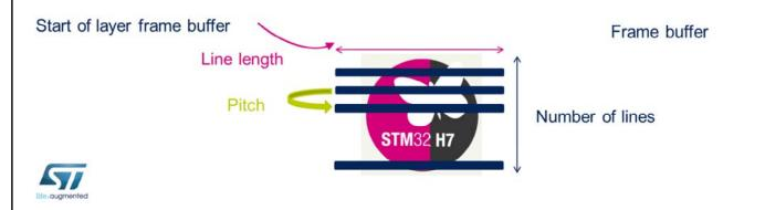
Every layer has configurable number of lines and line length for the color frame buffer and the pitch.
