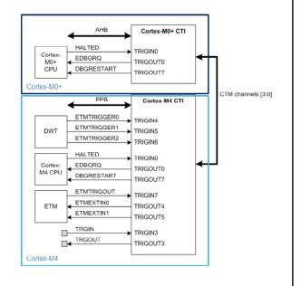
Cross triggering can be used in dual-core devices to halt both cores simultaneously. When one core hits a breakpoint, its "halted" output (indicating it has entered debug mode) propagates to the other core and causes it to enter debug mode as well. Similarly, both cores can restart simultaneously.
