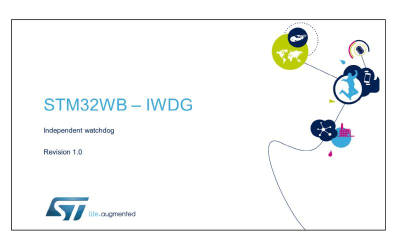
Hello and welcome to this presentation of the STM32 independent watchdog (IWDG). It covers the main features of this peripheral which can be used either as a watchdog to reset the microcontroller when a problem occurs, or as a free-running timer for application timeout management.
