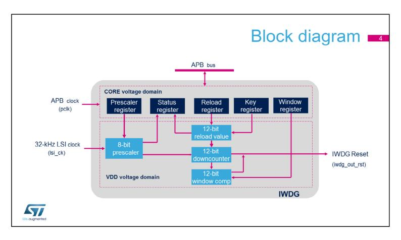
The independent watchdog registers are located in the CORE voltage domain while its functions are in the VDD voltage domain.
