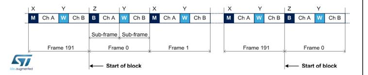
In IEC60958 specifications, the block structure is used to decode the Channel Status (CS), and User information (U).
