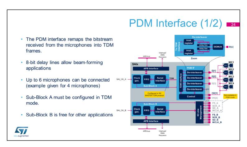
The PDM interface remaps the bitstream received from the digital microphones into TDM frames.
