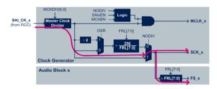
f<sub>FS</sub> is the sampling rate frequency (~ frame period) f<sub>SCK</sub> is the bit clock frequency
