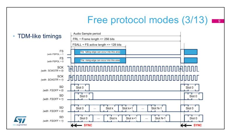
The following example shows some of the possibilities of the interface for the TDM-like protocols. In a TDM-like protocol:
