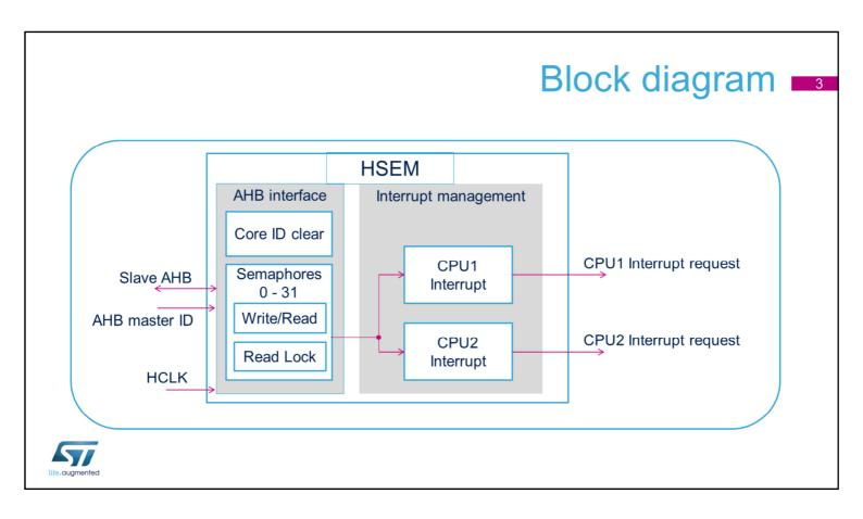
The HSEM module is located on the AHB bus. It consists of an "AHB interface" containing the semaphores and an "Interrupt management" block handling the interrupt distribution.
