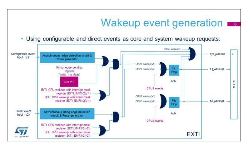
The CPUs wakeup signals generated by the EXTI block are connected to the PWR block, and are used to wake up the system and CPU sub-systems bus clocks.
