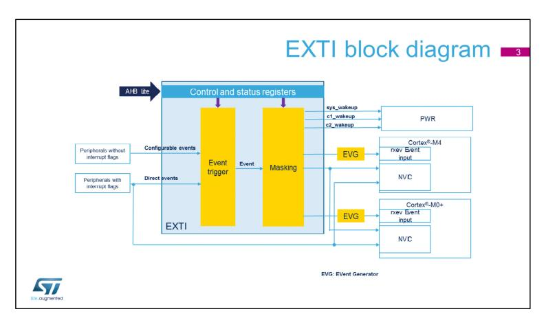
This is the block diagram of the extended interrupt and event controller.
