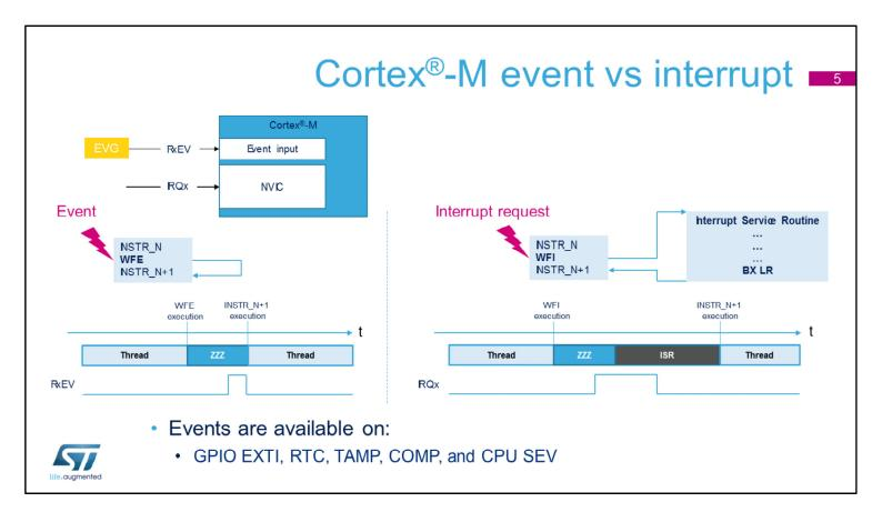
The Cortex®-M supports two ways to enter a low-power state:
