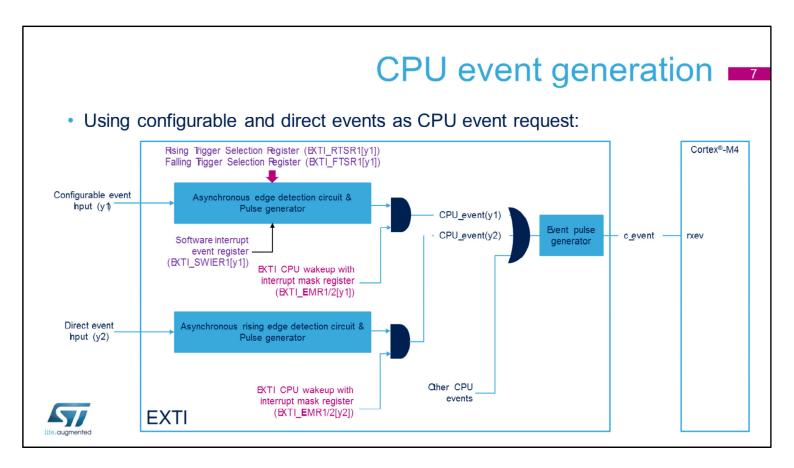
This figure aims to explain the various stages enabling the conversion of a configurable event active edge into a processor event.
