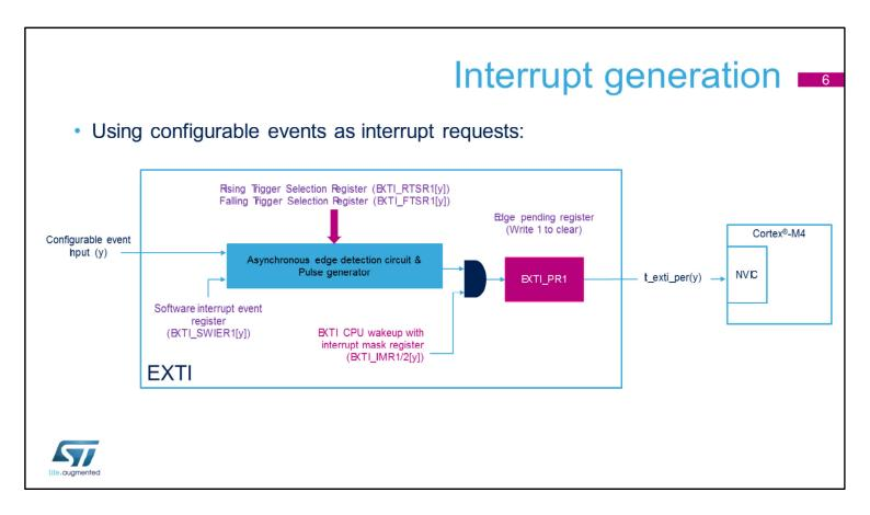
This figure aims to explain the various stages enabling the conversion of a configurable event active edge into an interrupt request.
