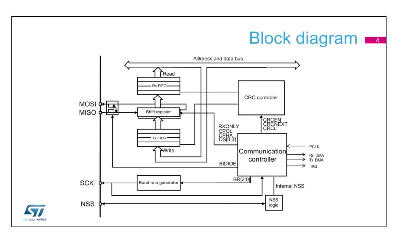
The simplified SPI block diagram shows the basic control mechanisms and functions. There are 4 I/O signals associated with the SPI peripheral. All of the data passes through receive and transmit buffers via their specific interfaces. The control block features are enabled or disabled depending on the configuration.
