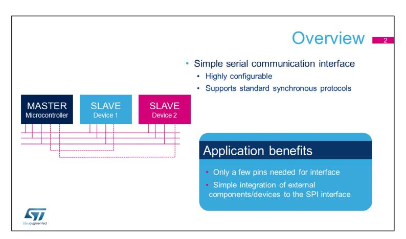
The internal Standard Peripheral Interface or SPI provides simple communication interface allowing the microcontroller to communicate with external devices. This interface is highly configurable to support many standard protocols. Applications benefit from the simple and direct connection to components which requires a few pins. Thanks to the highly configuration capabilities of the SPI, many devices can be simply accommodated in the existing project.
