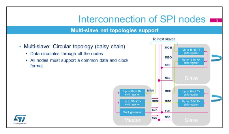
Another multi-slave configuration is the circular topology where the inputs and outputs of all the nodes are connected together in a closed serial chain. A common Slave Select signal is used for all the nodes as communication occurs at the same time. All nodes must have the same data and clock format configuration. Microcontroller SPI nodes typically use separate internal transmit and receive shift registers, so the data transferred between them has to be handled by software in a circular mode.
