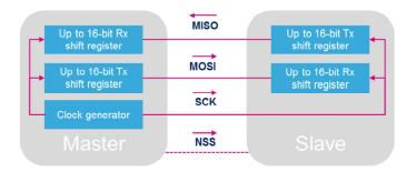
In Full-duplex mode (bidirectional), both master and slave transmit and receive data at the same time
