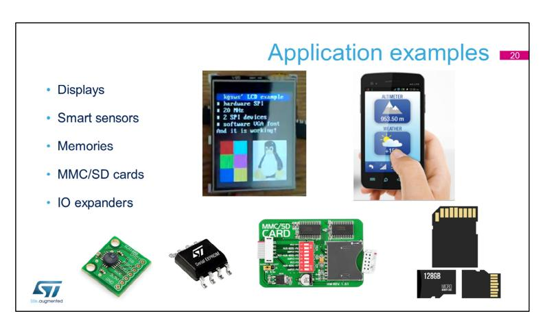
The SPI can be used in a wide range of applications where a simple data transfer is required without the need for a complex communication protocol. Secured transfers are also supported when used with smart cards.
