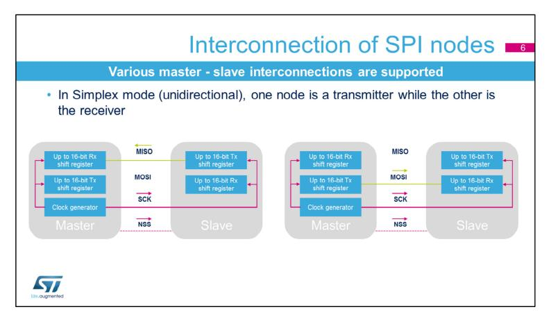
In Simplex mode, one node transmits data while the other receives the data. Data only flows in one direction. Depending on the communication direction, only one data line is used. Unused SPI pins can be used for other purposes.
