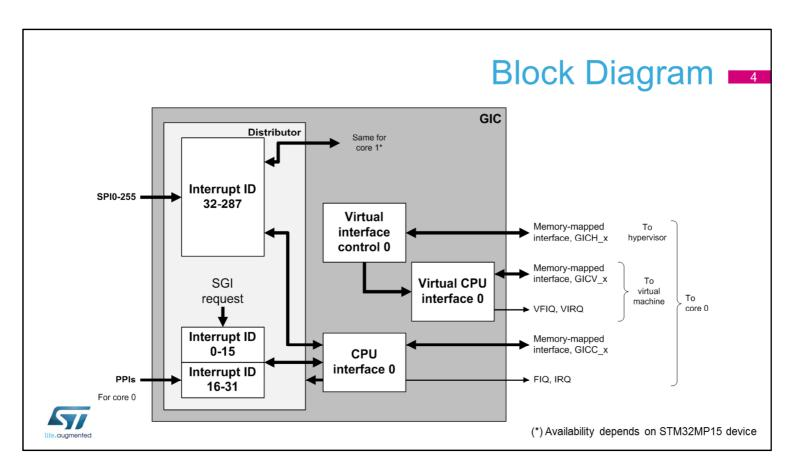
The GIC receives up to 256 interrupts from STM32MP15 peripherals shared between the two Cortex-A7 cores. In addition, up to 16 internal private peripheral interrupts (PPI) and up to 16 software generated interrupts (SGI) are managed by each Cortex-A7 core.
