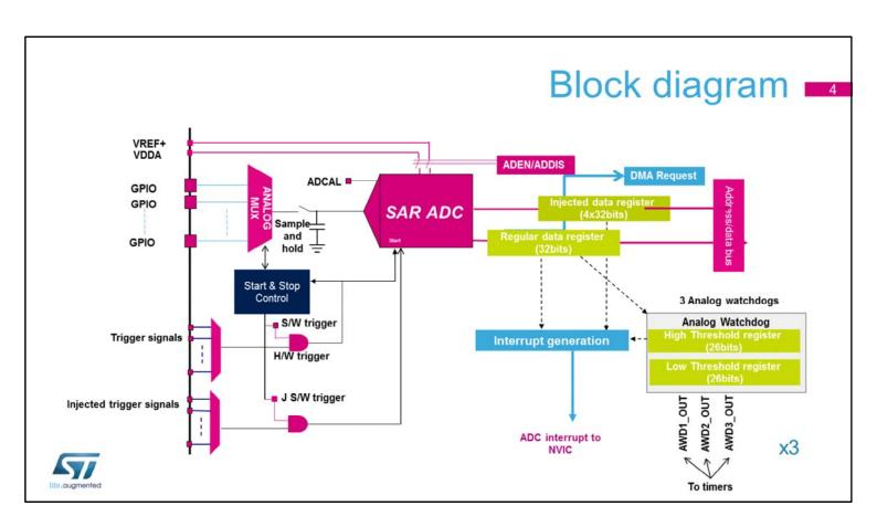
This slide shows the general block diagram for the 3 analog-to-digital converters embedded in the STM32H7.
