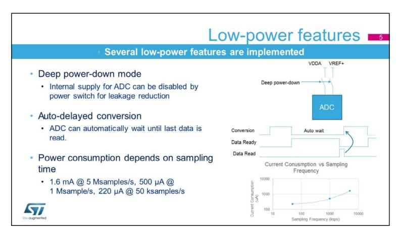
The STM32H7's ADCs support a Deep power-down mode. When the ADC is not used, it can be disconnected by a power switch to further reduce the leakage current. Autodelayed mode makes the ADC wait until the last conversion data is read before starting the next conversion. This avoids unnecessary conversions and thus reduces power consumption. The power consumption is in function of the sampling frequency. For low sampling rates, the current consumption is reduced almost proportionally.
