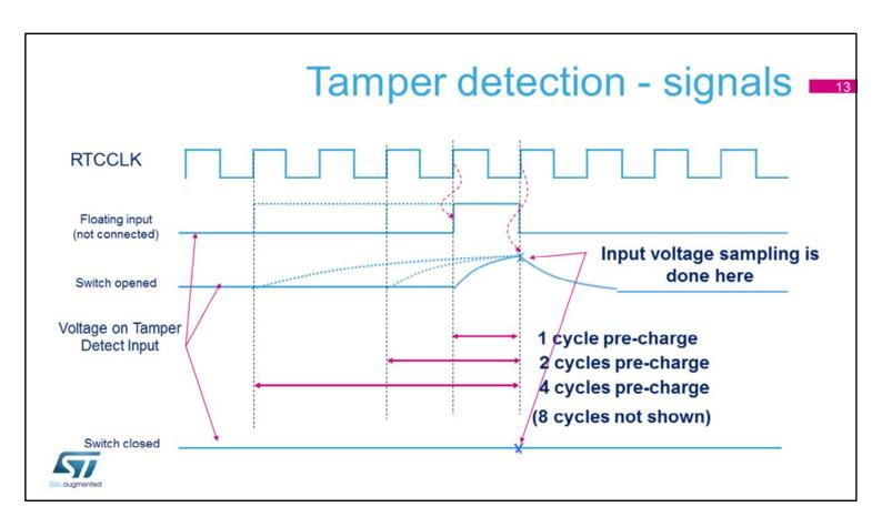
This figure illustrates tamper detection using the internal pull-up. The internal pull-up can be applied for 1, 2, 4 or 8 cycles. If the switch is opened, the level is pulled-up by the resistor. If the switch is closed, the level remains low. The input voltage is sampled at the end of the pre-charge pulse.
