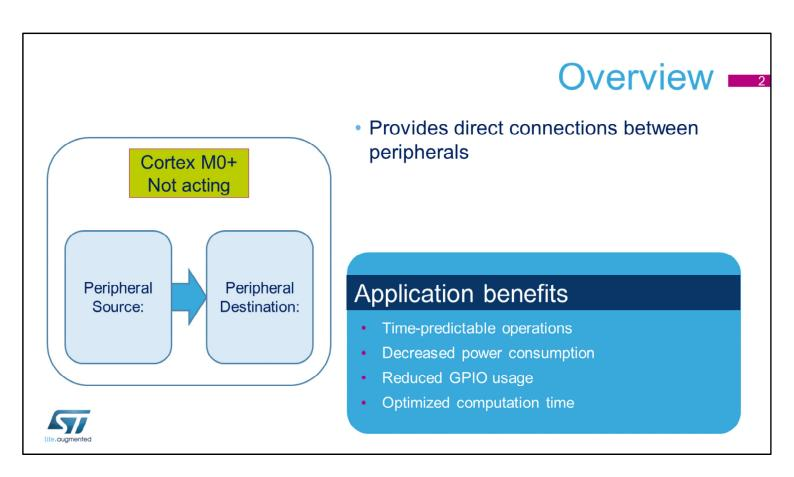
The Interconnect Matrix integrated inside STM32 products provides direct connections between peripherals.
