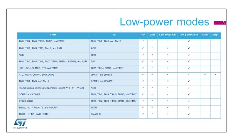
Peripherals can be interconnected using the Interconnect Matrix even when the circuit is in a low-power mode. This table indicates in which low-power modes, the interconnection between peripherals remains active.
