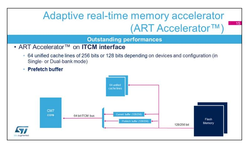
The ART accelerator is available only on the Cortex-M7 ITCM interface. It brings outstanding performance and reduces cache usage while executing code from Flash memory. It consists of 64 unified cache lines with a 256-or 128-bit width depending on the Flash memory interface width configuration. For each Cortex-M7 fetch a lookup in current buffer, prefetch buffer and ART cache is performed. If there is a hit, the data is immediately returned to the CPU.
