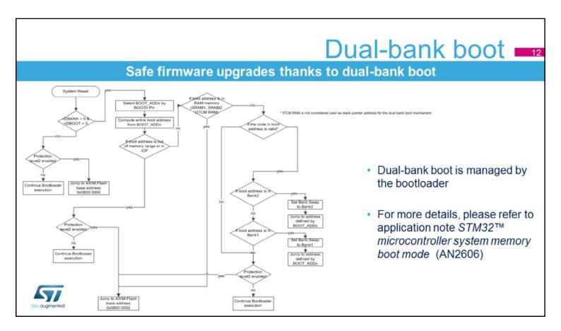
The dual-bank boot allows a safe firmware upgrade as the previous firmware version is still present in the other memory bank. The dual-bank boot is managed by the bootloader. The device boots in Bank 2 using the nDBOOT option bit, programmed in the Flash option bytes.
