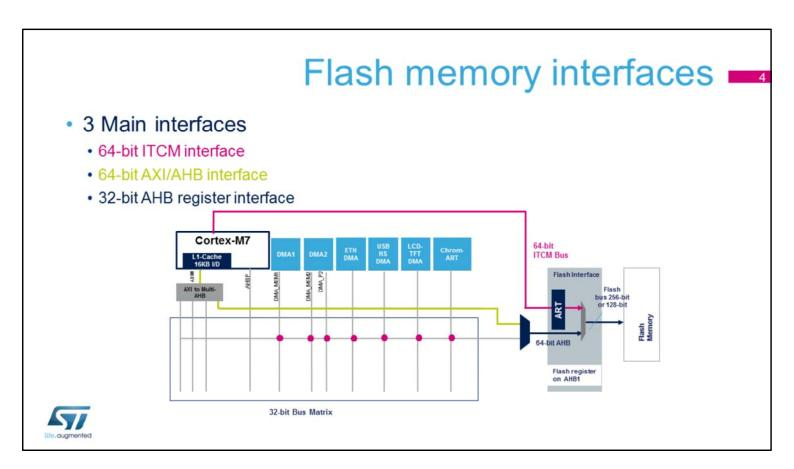
The Flash memory interface has three main buses, a 64-bit ITCM interface, a 64-bit AXI/AHB interface and a 32-bit AHB register interface.
