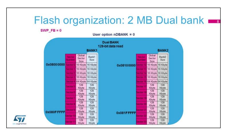
In Dual-bank mode (for STM32F76x/F77x MCUs), the 2 Mbytes of Flash memory is organized as 12 sectors for each Flash memory bank. Where each bank has 4 sectors of 16 Kbytes, one sector of 64 Kbytes and 7 sectors of 128 Kbytes. Bank 2 sectors start from sector 12 to sector 23.
