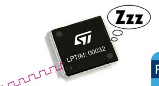
The LPTIM is a 16-bit timer. Thanks to its diversity of clock sources, the LPTIM is able to keep running in most of the available lowpower modes of the STM32H7 microcontroller.
