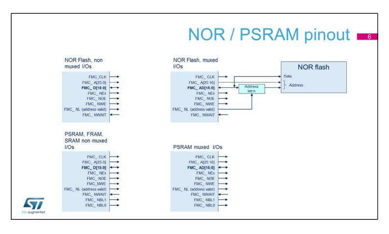
The flexible memory controller supports non-multiplexed and multiplexed PSRAM, FRAM, SRAM and NOR interfaces.
