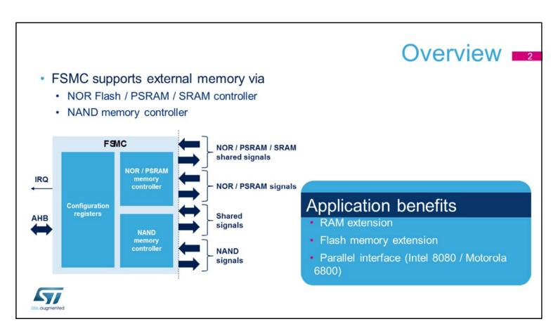
The FSMC controller integrated in STM32L5 products provides external memory support through two memory controllers: the NOR Flash, PSRAM and SRAM controller and the NAND memory controller. This enables the CPU to communicate with external memories including NOR and NAND Flash memories, PSRAM, and SRAM. This interface is fully configurable, allowing easy connection with external memories or other parallel interfaces.
