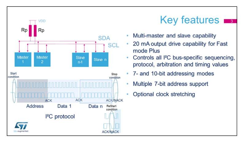
The I<sup>2</sup>C peripheral supports multi-master and slave modes. The I<sup>2</sup>C IO pins must be configured in open-drain mode. The logic high level is driven by an external pull-up. The IO pins support the 20 mA output drive required for Fast mode Plus. The peripheral controls all I<sup>2</sup>C bus-specific sequencing, protocol, arbitration and timing values.
