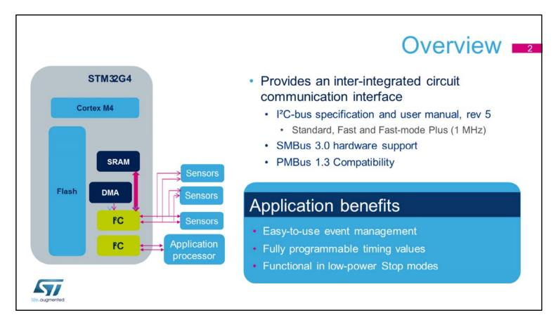
The I<sup>2</sup>C interface is compliant with the NXP I<sup>2</sup>C-bus specification and user manual, Revision 5; the SMBus System Management Bus Specification, Revision 3; and the PMBus Power System Management Protocol Specification, Revision 1.3.
