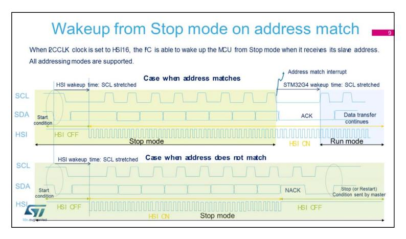
The I<sup>2</sup>C peripheral supports Wakeup from Stop mode on address matches. To do this, the I<sup>2</sup>C peripheral clock must be set to the HSI16 oscillator. Only the analog noise filter is supported when the Wakeup from Stop feature is enabled. All addressing modes are supported.
