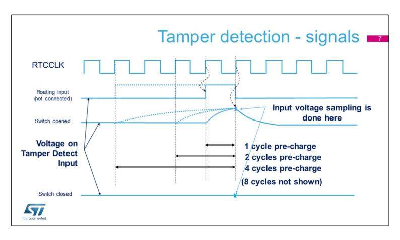
This figure illustrates tamper detection using the internal pull-up.
