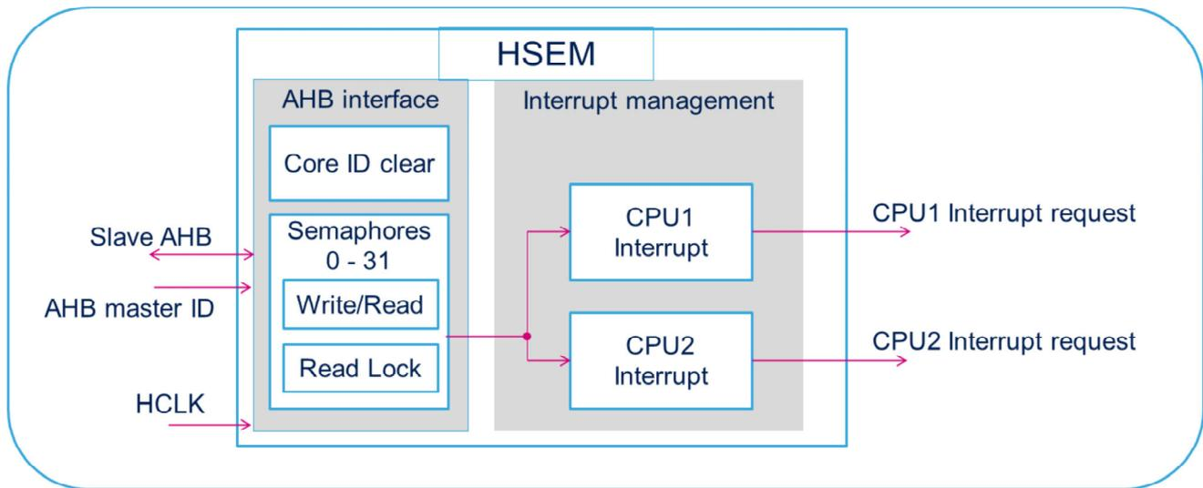
The HSEM module is located on the AHB bus. It consists of an “AHB interface” containing the semaphores and an “Interrupt management” block handling the interrupt distribution.
