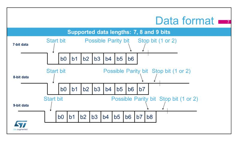
The frame format consists of a set of data bits in addition to bits for synchronization and optionally a parity bit for error checking. A frame starts with one start-bit (S), where the line is driven low for one bit-period. This signals the start of a frame and is used for synchronization.
