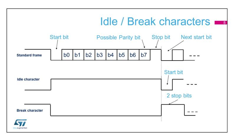
The previous slide described a standard frame. This slide shows an example of an 8-bit data frame configured with 1 stop bit.
