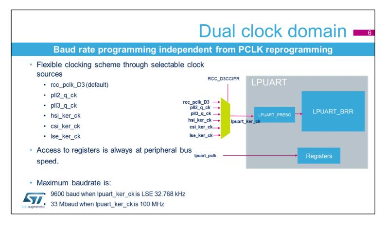
Its clock source can be selected in the RCC, and can be either the peripheral clock (APB clock), the PLL2\_q, the PLL3\_q, the HSI, CSI or LSE clock.
