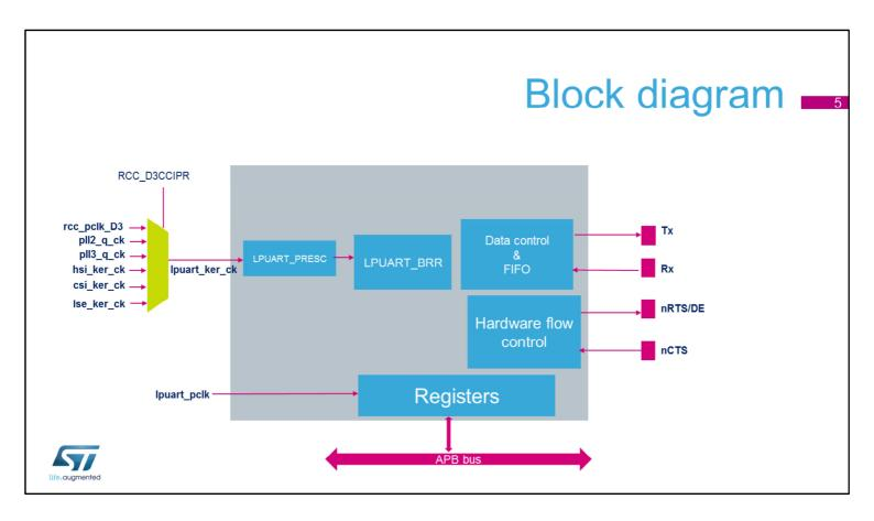
Here is the LPUART block diagram. The LPUART clock "lpuart\_ker\_ck" can be selected from several sources: peripheral clock (APB clock), the PLL2\_q, the PLL3\_q, the high-speed internal RC oscillator or the low-power internal oscillator (CSI) or the low-speed external 32.768 kHz crystal oscillator (LSE).
