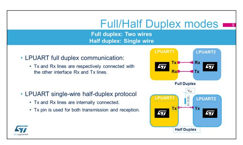
The LPUART supports full-duplex communication where the Tx and Rx lines are respectively connected with the other interface's Rx and Tx lines.
