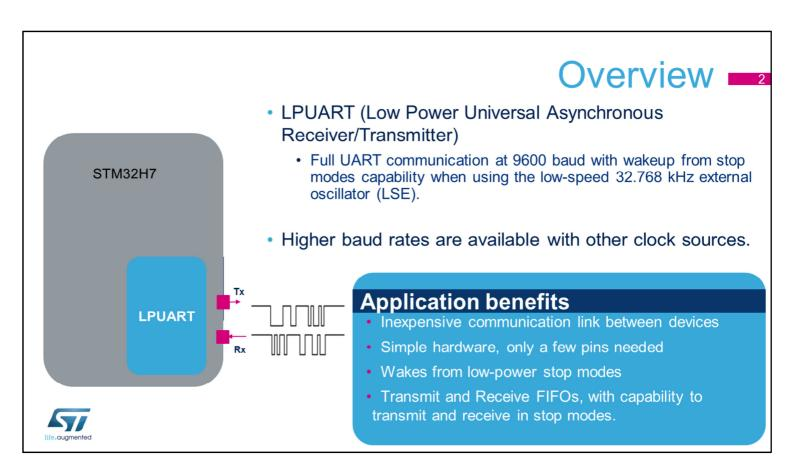
The Low Power Universal Synchronous Asynchronous Receiver provides full UART communications at 9600 baud when the LPUART is clocked using a low-speed external 32.768 kHz oscillator (LSE).
