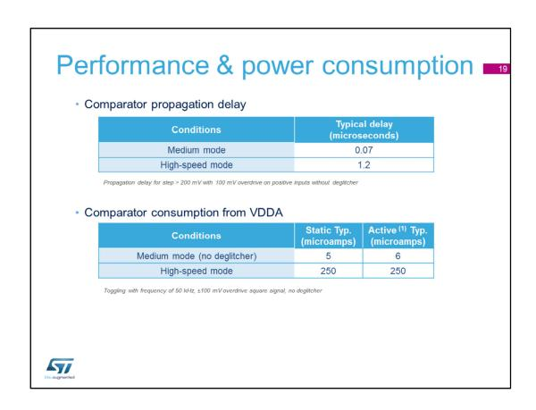
The on-chip comparator configuration capability allows the user to select the best performance point for the targeted application. It replaces the external stand-alone comparator, thereby reducing the bill of materials.
