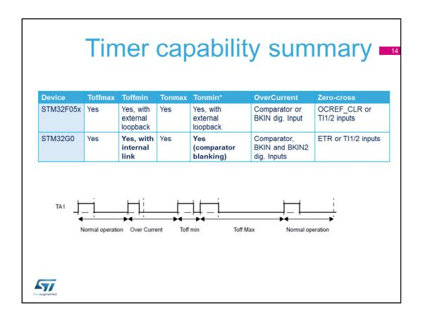
When combined with a PWM output from a timer, the cycle-by-cycle current control loop is simplified in the STM32G0 with regard to STM32F0 microcontrollers. No external loopback is required.
