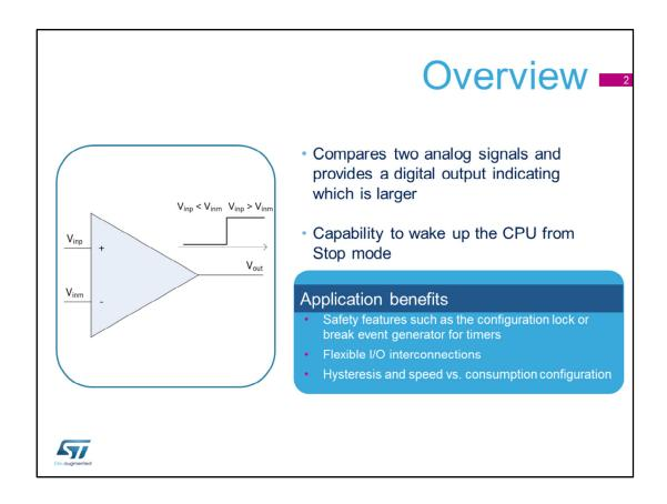
The two analog comparators inside STM32 microcontrollers provide a binary output which indicates if the analog voltage on the plus input is larger than the voltage on the negative input. It allows the MCU to react when the analog signal crosses a predefined threshold. The comparator continuously monitors voltage in contrast to an analog-to-digital converter which operates in sampled mode.
