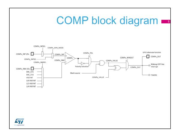
This slide shows the general block diagram of the comparator integrated in STM32G0 microcontrollers.
