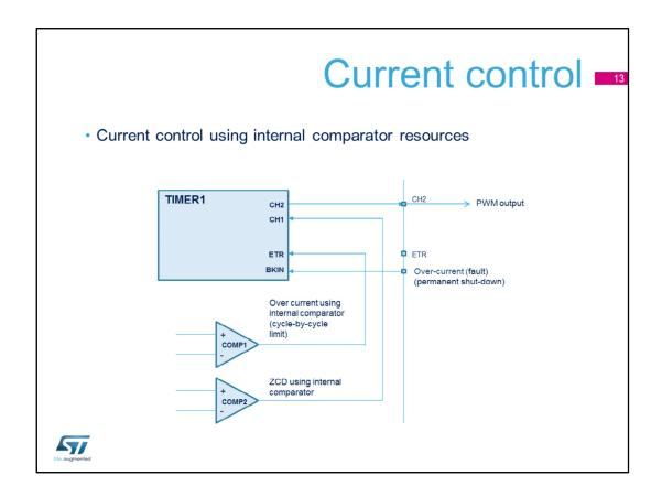
The figure represents an example of direct connection between Timer and COMP units.
