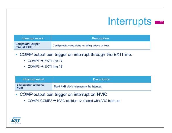
The comparator can trigger an interrupt on the rising, falling or both edges of the comparator output through the EXTI line. This is required to exit the Stop modes. The output can also be connected to the CPU's nested vectored interrupt controller (NVIC).
