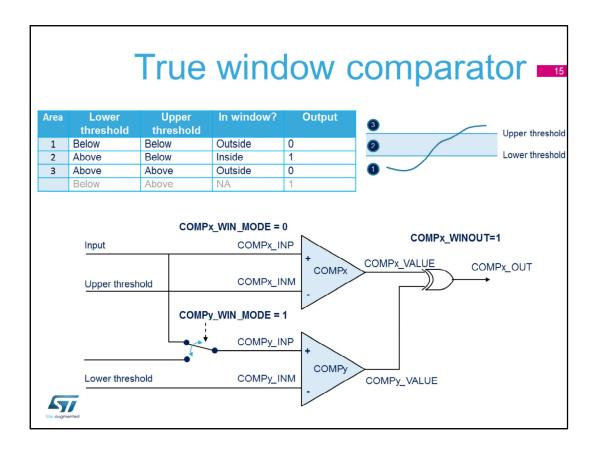
The purpose of the window comparator is to trigger an interrupt if the analog voltage exceeds the predefined lower and upper voltage thresholds applied to the inverting inputs of each comparator. This event can generate an interrupt through the EXTI line. Two non-inverting inputs can be connected internally by enabling the WINMODE bit and therefore save one IO for another purpose.
