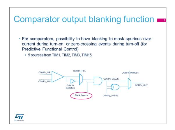
The blanking function aims to mask the output of the comparator during period of times indicated by a timer. This is typically used in the PFC technique (Predictive Functional Control).
