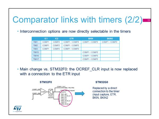
The upper table is the connection matrix between the comparator and the timer units.
