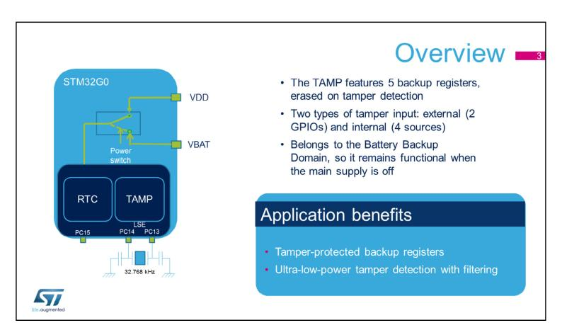
The TAMP peripheral features five 32-bit backup registers used to preserve data when the main supply is off. These backup registers can be used to store secure data, as they are erased when a tamper event is detected on the tamper pins or on some internal events. The tamper detection is functional in low-power modes when the VBAT domain is supplied by a backup battery. The anti-tamper circuitry includes ultra-low-power digital filtering, avoiding false tamper detections.
