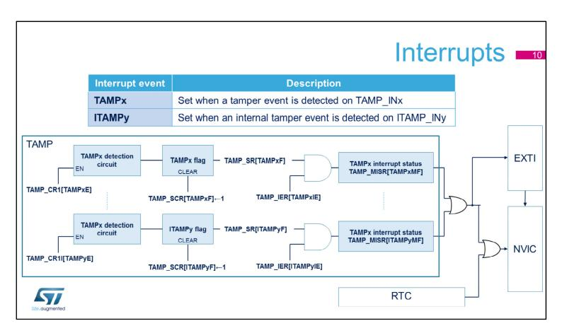
All interrupts can wake the processor up from all low-power modes. The detection on all tamper pins and internal tamper sources can generate an interrupt. Any tamper detection circuit can be enabled or disabled by programming the TAMP\_CR1 register. If it is enabled and a tamper event is detected, the corresponding flag is set in the TAMP\_SR register. Then TAMP\_IER register masks or enables the tamper event interrupt.
