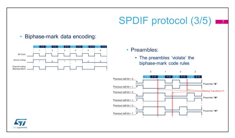
The digital audio data are coded using biphase-mark encoding as shown in the upper figure.
