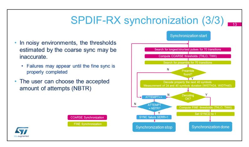
The figure shows the hardware process performed by the SPDIF\_RX in order to estimate properly the THLO and THHI thresholds.
