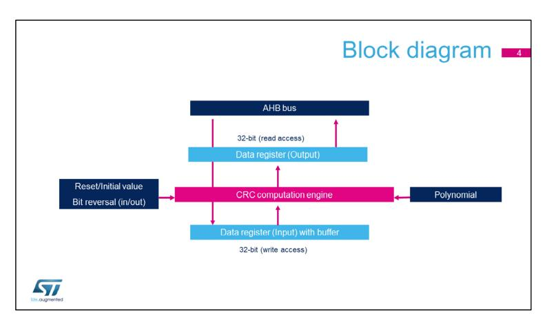
The CRC calculation unit is connected to the AHB bus interface for an optimal performance.
