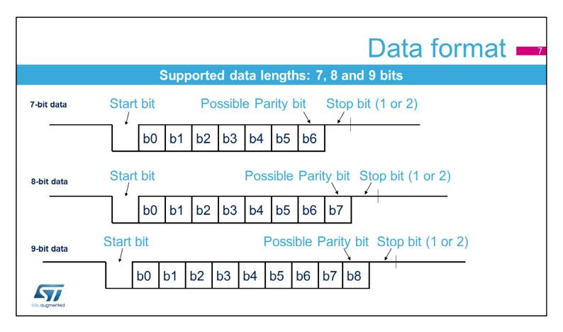
The frame format consists of a set of data bits in addition to bits for synchronization and optionally a parity bit for error checking. A frame starts with one start-bit (S), where the line is driven low for one bit-period. This signals the start of a frame and is used for synchronization.
