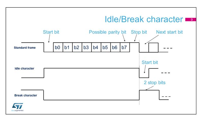
The standard frame was described in the previous slide. This slide shows an example of 8-bit data frames configured with 1 stop bit.
