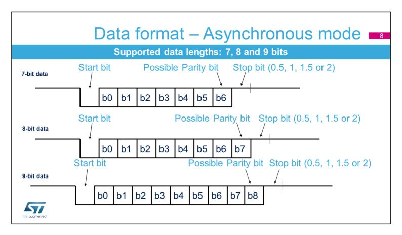
The frame format used in Asynchronous mode consists of a set of data bits in addition to bits for synchronization and optionally a parity bit for error checking.
