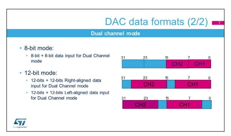
In Dual channel mode, it's an 8-bit plus 8-bit data format, in order to provide input data for two DAC simultaneously. In 12-bits + 12-bits, either a right- or left-aligned mode can be used for input data.
