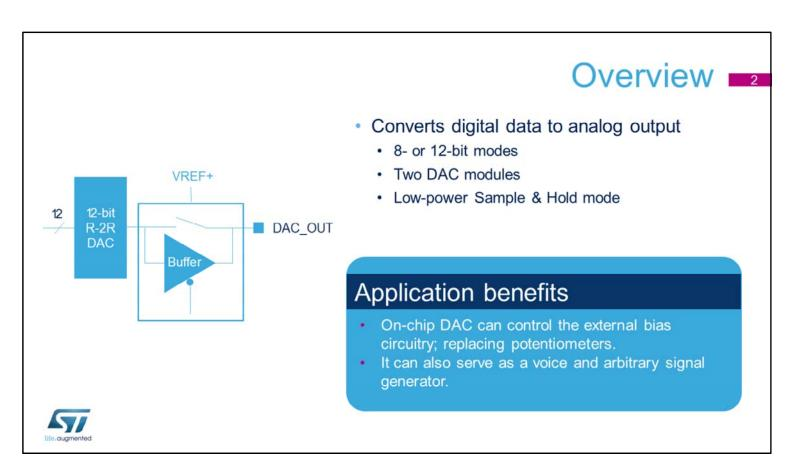
The STM32MP1 digital-to-analog converter converts 8or 12-bit digital data to an analog voltage. Two DAC modules are embedded in the **STM32MP1 microprocessor.**
