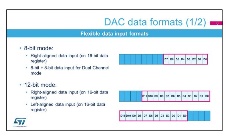
The DAC can support different input formats. In 8-bit mode, it's a right-aligned 8-bit data format.
