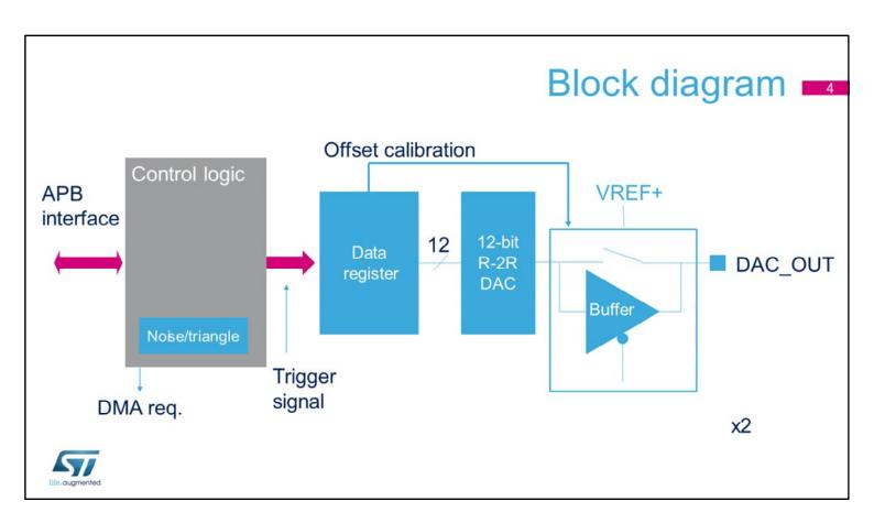
Here you can see the simplified block diagram of the digital-to-analog converter. The STM32MP1 integrates 2 of them. The block DAC is supplied by VDDA.
