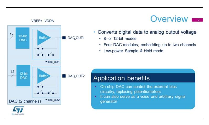
The STM32G4 digital-to-analog converters converts 8- or 12-bit digital data to an analog voltage.
