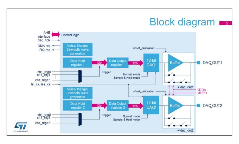
Here you can see the simplified block diagram of the digital-to-analog converter.
