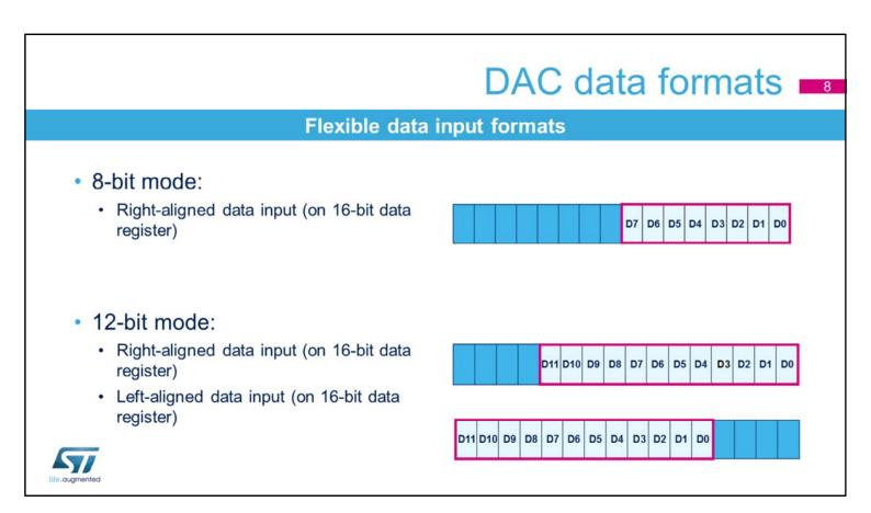
The DAC can support different input formats. In 8-bit mode, it is a right-aligned 8-bit data format. It also accepts the unsigned and signed data format.
