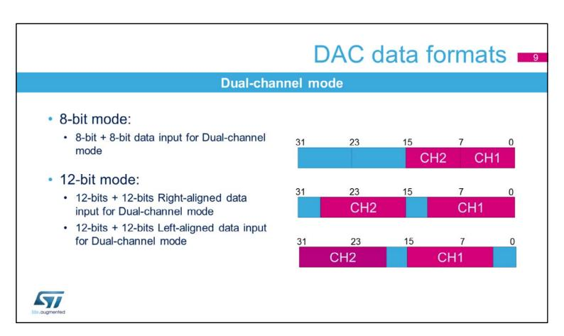
In Dual-channel mode, it is an 8-bit plus 8-bit data format, in order to provide input data for two DACs. In 12-bits + 12-bits, either a right- or left-aligned mode can be used for input data.
