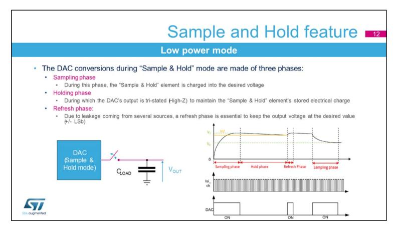
The digital-to-analog converter can work intermittently, charge the external or internal capacitor, and be powered down while the output voltage is kept on the hold capacitor. After the refresh period, the DAC is powered back on again and recharges the hold capacitor.
