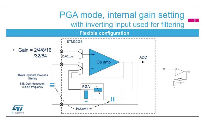
The op amps also support external connections on outputs and the inverting input for the PGA mode. It enables the connection of an external capacitor to add low-pass filter characteristics to the PGA configuration.
