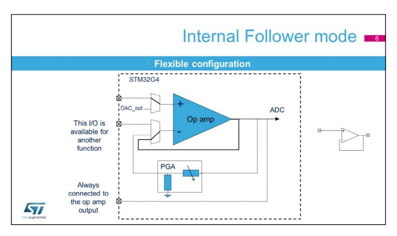
The operational amplifiers can be configured as an internal voltage follower, where the internal switch connects the output to the inverting input. In internal voltage follower mode, the GPIO pad assigned to the op amp's inverting input can be free, so that it may be used with a different functions as subsequently assigned in the GPIO selection process.
