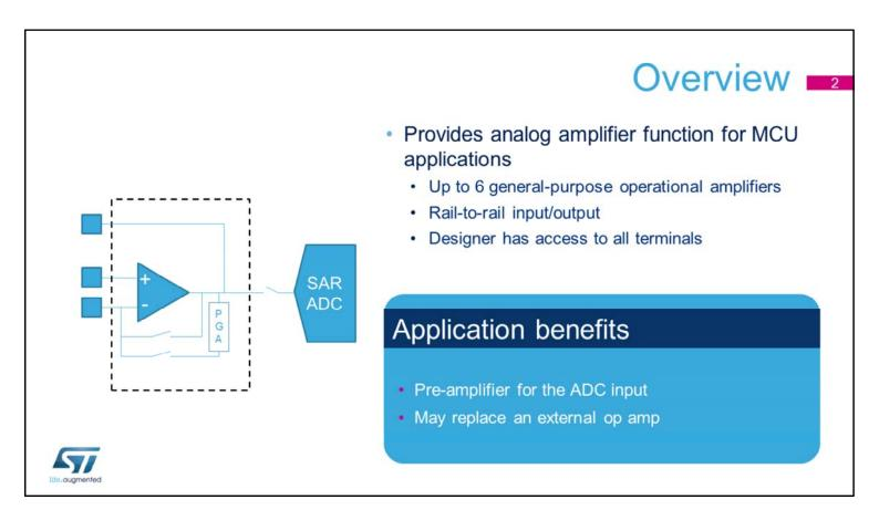
Up to four operational amplifiers inside STM32G4 products functions as a general-purpose analog amplifier, which may reduce the need for an external stand-alone op amp. As these op amps can be configured in stand-alone mode with all terminals available for the user, it is possible to use them as a voltage follower, non-inverting and inverting amplifiers, as well as analog filters such as low- or high-pass filters. They can also act as a pre-amplifier for the ADC input.
